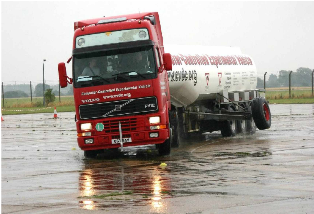
40 tonne articulated truck being driven around a circular path using the ABD path following system
